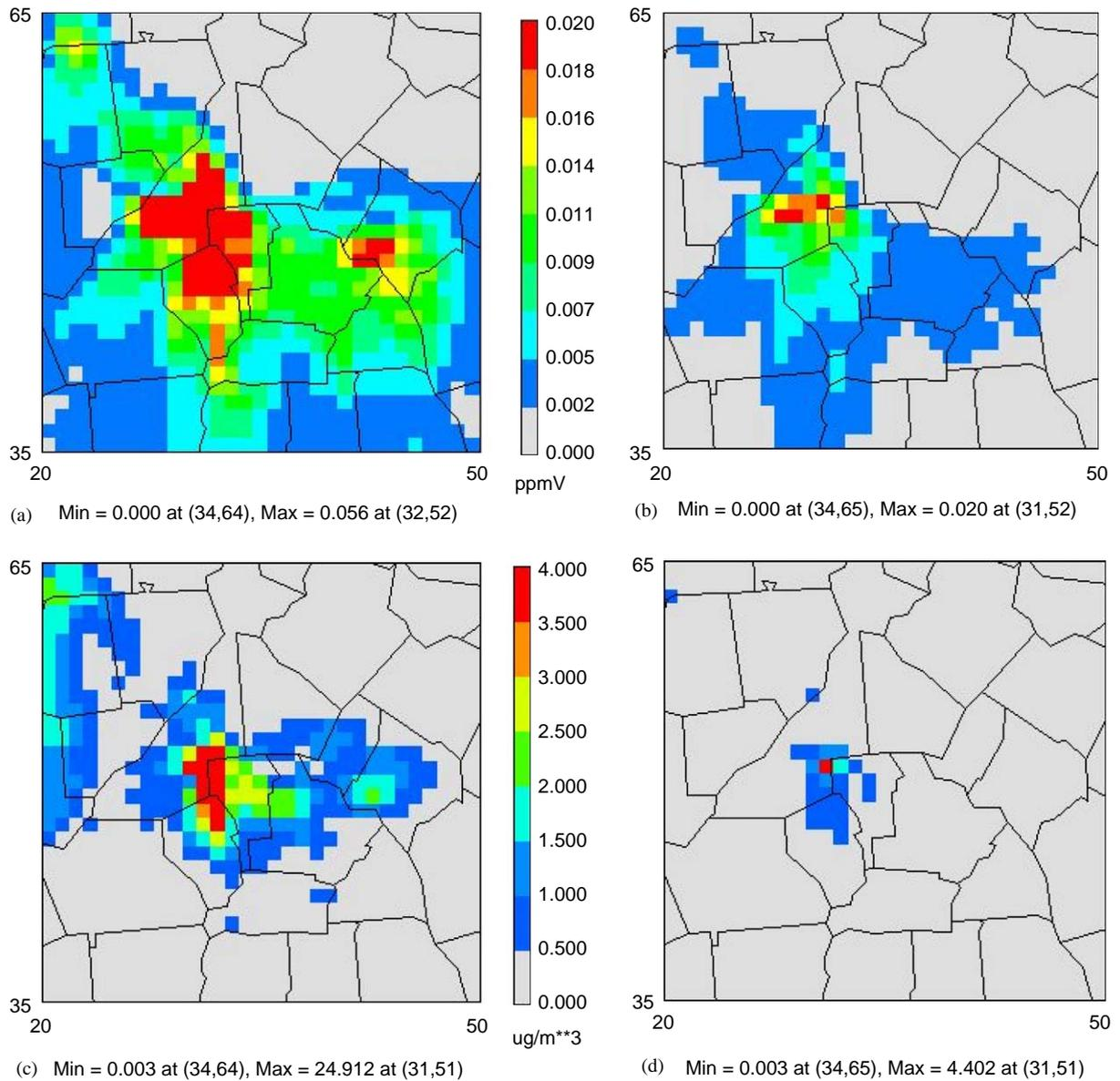
Fig. 4. Maximum sensitivity of regional concentrations to aircraft emissions from Hartsfield–Jackson Atlanta International Airport during the August 11–20, 2000 period: (a) O<sub>3</sub> to characteristic value emissions; (b) O<sub>3</sub> to mode specific emissions; (c) PM<sub>2.5</sub> to characteristic value emissions; and (d) PM<sub>2.5</sub> to mode specific emissions.
