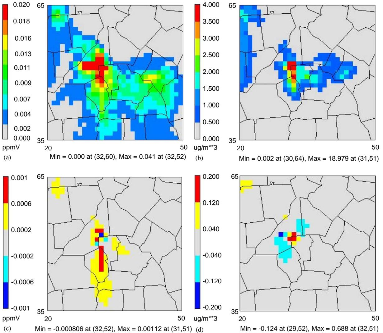
Fig. 6. Difference of injecting aircraft emissions (mode specific) into the first-layer airport cells from distributing them in 3-D space: (a) maximum O<sub>3</sub>; (b) maximum PM<sub>2.5</sub>; (c) average O<sub>3</sub>; (d) average PM<sub>2.5</sub>.
