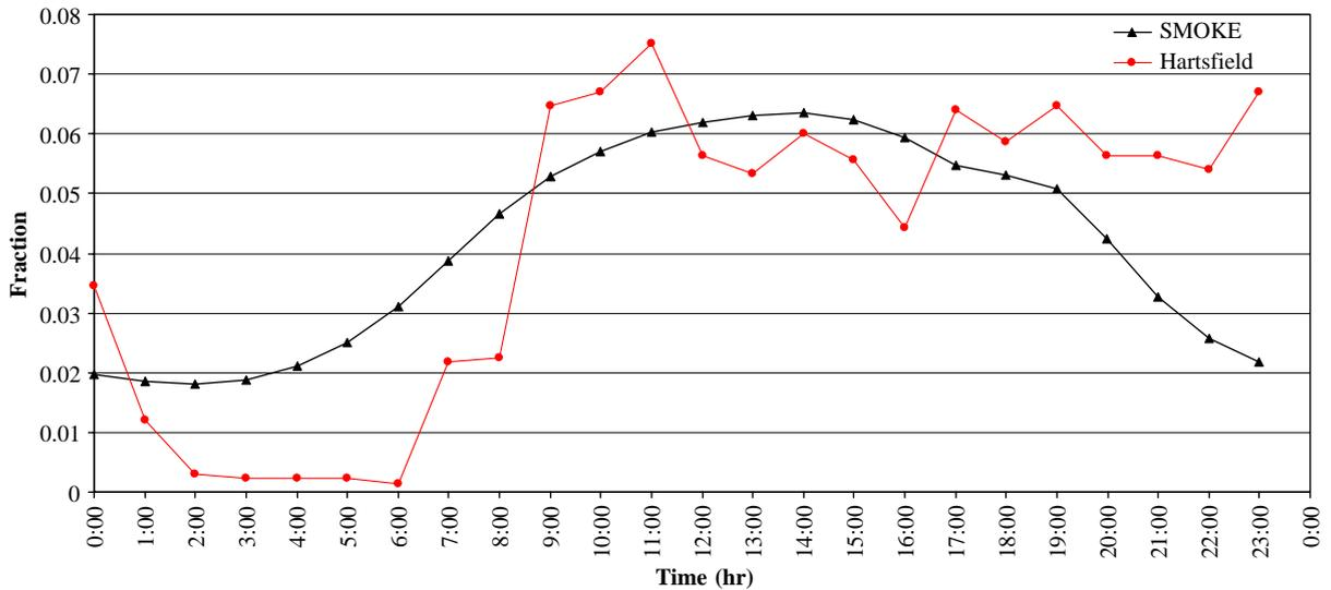
Fig. 2. Diurnal flight activity profile for Hartsfield–Jackson airport and the default profile used in SMOKE for commercial aircraft (SCC = 227502000).
