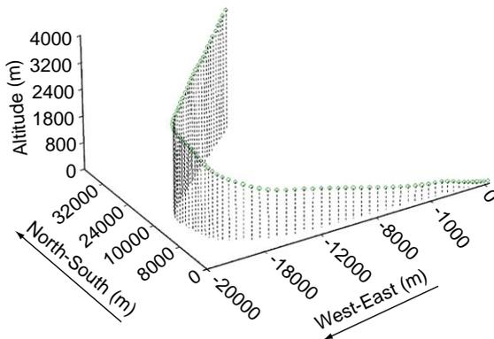
Fig. 3. Typical 3-D path for DC-9s for takeoff and climb-out modes at Atlanta Hartsfield–Jackson airport in August 2000 (Zero indicates the location where the runway ends).
